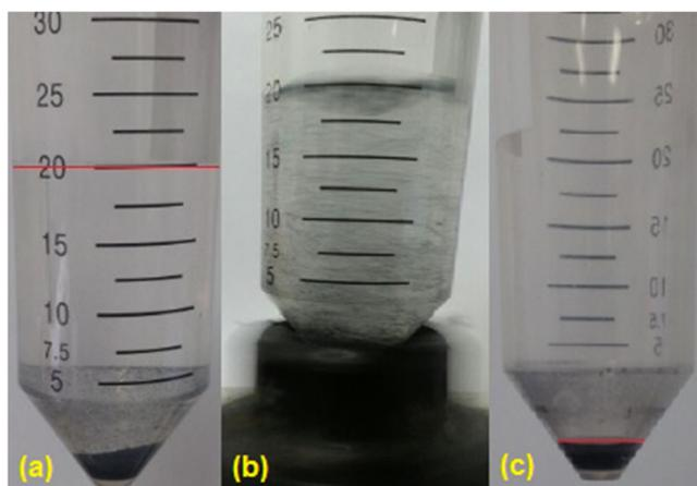
**Fig 1** Photographs of COU-2-D- $\mu$ -SPE: **a** COU-2 in sample solution, **b** extraction of analytes using vortex system, and **c** desorption of analytes from the COU-2 sorbent (horizontal lines indicate the levels of solutions)
