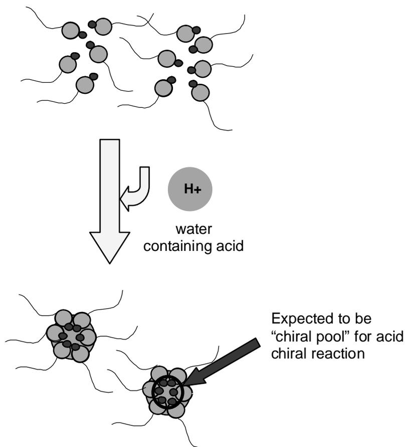
Figure 9 Amphiphilic chiral solid catalyst as heterogeneous micellar catalyst in enantioselective hydration of epoxycyclohexane<sup>[31]</sup>
