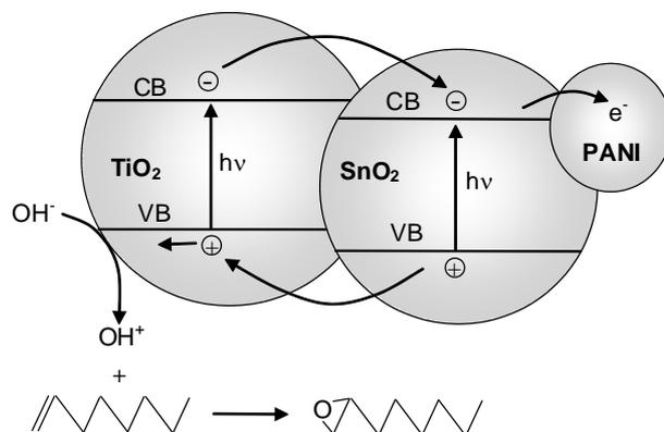
Figure 7. The proposed mechanism of photocatalytic epoxidation of 1-octene over PANI-SnO<sub>2</sub>-TiO<sub>2</sub><sup>[29]</sup>
