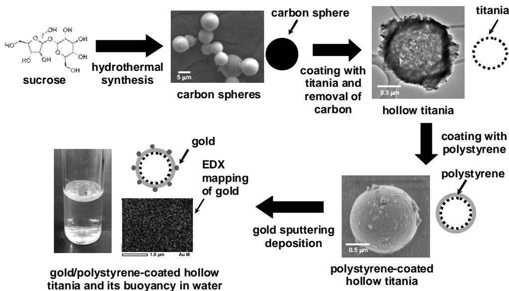
Figure 4. Schematic illustration of floating gold/PS-HT synthesis procedure with TEM micrograph of hollow titania, FESEM micrographs of CS and PS-HT<sup>[19]</sup>
