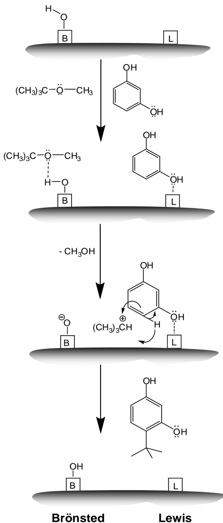
Figure 8. Proposed mechanism of the alkylation of resorcinol with MTBE<sup>[30]</sup>
