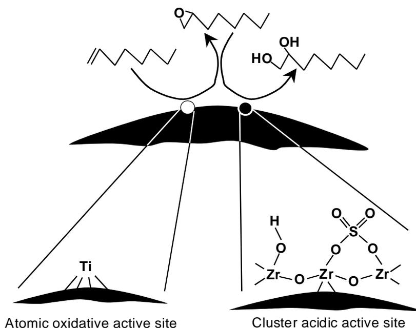
**Figure 6. Proposed model of TS-1 loaded with sulfated zirconia as bifunctional catalyst for consecutive transformation of 1-octene to 1,2-octanediol through the formation of 1,2-epoxyoctane<sup>[24]</sup>**
