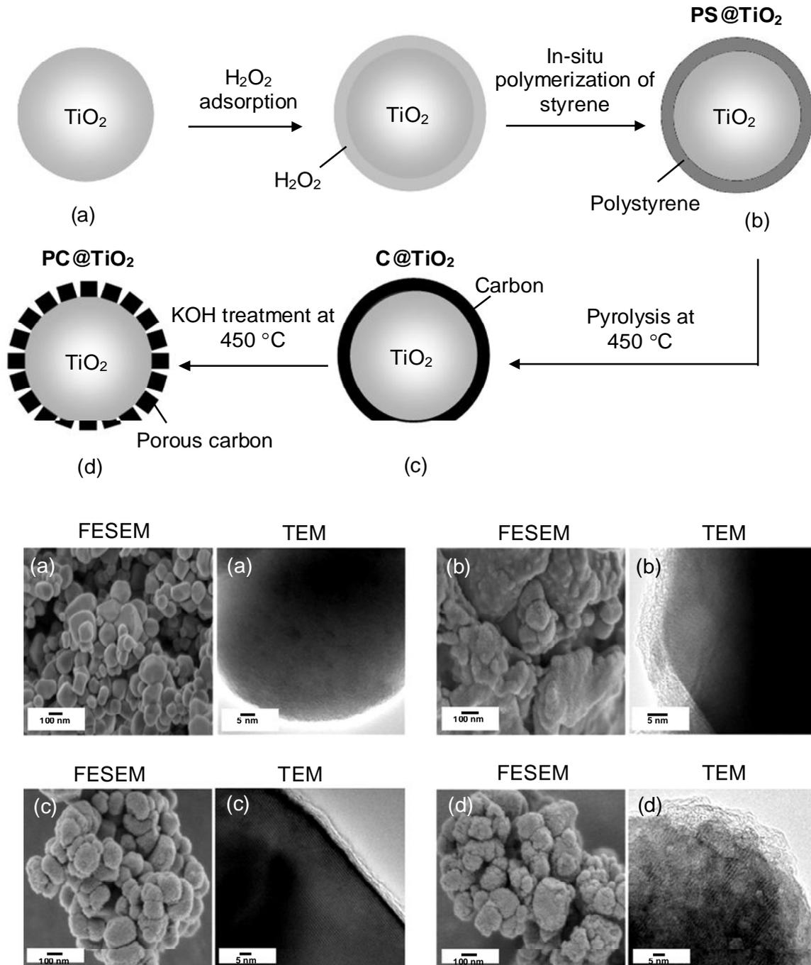
Figure 5. Schematic diagram of the preparation of PS@TiO<sub>2</sub>, C@TiO<sub>2</sub> and PC@TiO<sub>2</sub> particles and their FESEM and TEM photographs<sup>[20]</sup>
